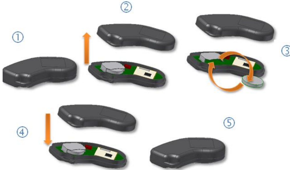
Figure 3 : procedure for a battery change
